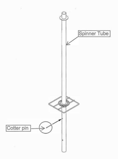
(2) Insert spinner tube through a spinner platform. Note orientation of spinner platform. Raise the spinner platform up and fully insert the cotter pin into the indicated hole. Lower the spinner platfom so that it rests on the cotter pin.
