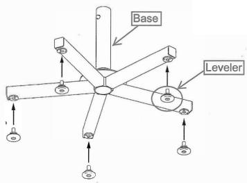
1) Screw all 5 levelers into the bottom of the base.
