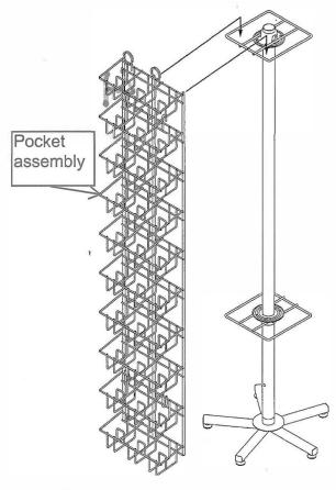
(5) Drop the top hooks of the pocket assembly onto the top spinner platform.
