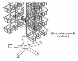
Remove cotter pin from lower spinner platform.
