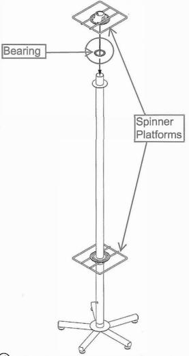
Place bearing on spinner tube washer and rest spinner platform on top of bearing.
